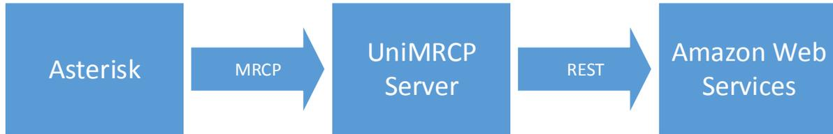
Note that the Asterisk and the UniMRCP server typically reside on different hosts in a LAN, although both might be installed on the same host.
